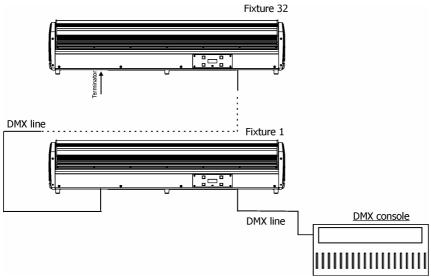
Caution: Terminate the link by installing a termination plug in the output of the last fixture. The termination plug is a male 3-pin XLR plug with a 120 Ohm resistor soldered between Signal (–) and Signal (+).
