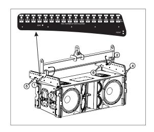
Once the first box is attached to the structure, the remaining boxes should be brought to the array and attached repeating the previous steps (1 and 2) using G1A50 guides and safety pins per side <u>making sure</u> that the pins have been inserted and locked correctly.
