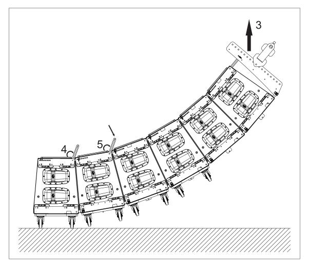
When the rear of the enclosures come together, the G2A48 rear guides should be positioned (4) into the hardware of the box above, inserting (5) the safety pins in the correct angle position. Since the boxes are flown, the safety pins should be in the slot of the G2A48 guide.
