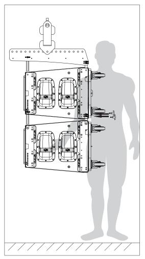
Once the boxes have been joined, the front dolly panels can be removed. The next boxes should be attached "one by one" using the methods described. Finally, the array should be hoisted to the correct height and secured with slings to avoid swinging.
