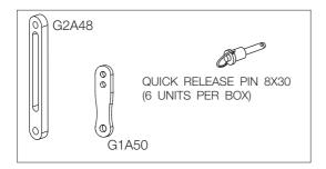
To aid the setting of the G2A48 guide in the corresponding hole in the top box, each hole is labeled with an associated angle, both for stacked and flown applications. To fit the guides into the holes, highly resistant 8 mm quick release pins with a ball safety lock are used.
