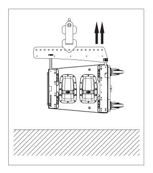
Once the first box has been placed at  $0^{\circ}$  and raised approximately 75cm (30 in) the second box of the array can be placed nearby. Once located in position, the G2A48 guides of the second box should be freed and inserted in the rear located receiving points of the suspended box and secured with the safety pins.
