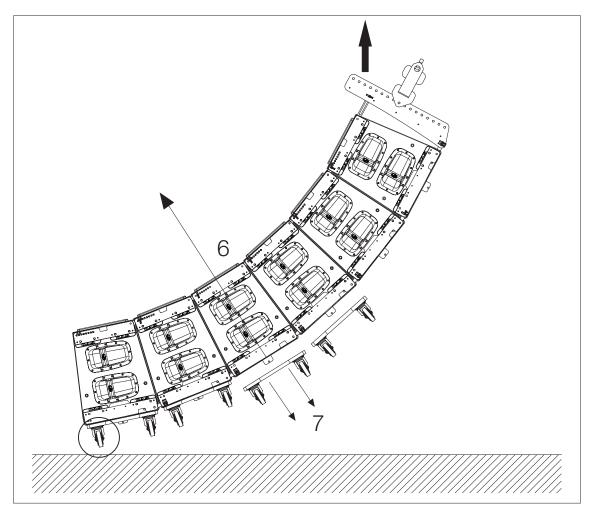
Once the complete array has been lifted into place, additional slings should be attached to secure the array and avoid swinging.
