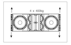
The maximum number of units that can be suspended from the AX-AERO50 flying grid is 16.
