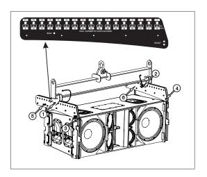
Once the first unit of the array has been attached to the AX-AERO50, the assembly should be lifted by way of the hoist until the wheels of the PL-50 dolly platform lift off the ground. From this point on, the hoist can be used to lift the box into a horizontal position.
