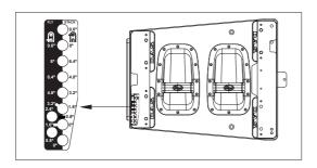
For flying boxes and defining the splay angle, the pins must be inserted in the slot of G2A48, whereas for stacking (stacked), the pin goes through the top hole of the guide.
