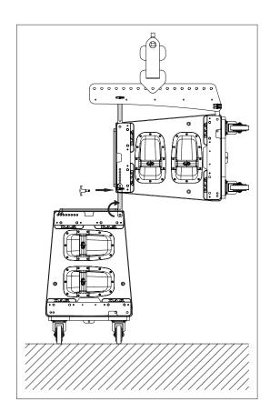
Once the splay angle between the first two boxes has been determined, the front of the box can be lifted into place. Three people will be needed to undertake this operation, two to lift the box and one to fit the G1A50 guide and safety pins into the upper box.
