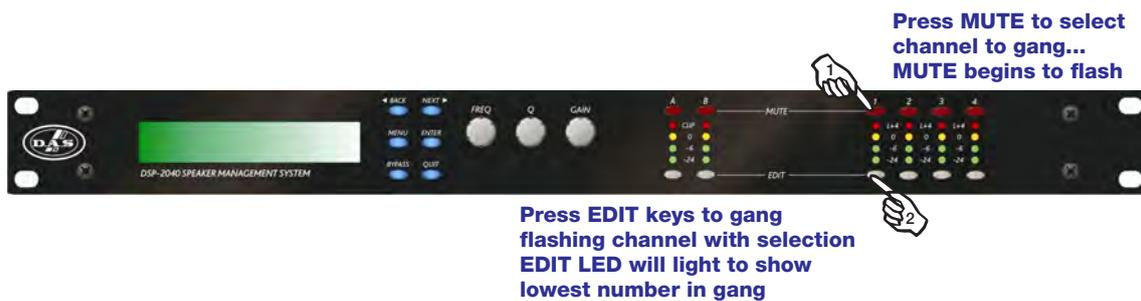
Press a MUTE key to choose the output to gang – its LED will begin to flash, and an EDIT key will illuminate to show which output it is currently ganged with. To change this selection, just press another EDIT key, remembering that gangs work from the highest to lowest number. So, to gang outputs 1 and 5, press MUTE 5 then EDIT 1 – the display will show
