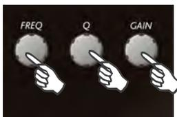
There are eight bands of parameter equalisation available on every input. The behaviour of each individual band can be changed to a variety of different filter shapes, including high and low shelves. Changing the filter type is achieved by pressing ENTER during editing any particular band. For more details about the various types of filter available, please see page 27.
