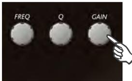
Use the GAIN allow to change its value. Pressing ENTER to confirm.
