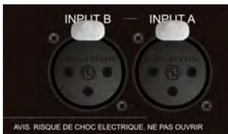
**[4]-Audio Inputs:** 3 pin XLR sockets are provided for each channel. All are fully balanced, pin 2 hot, 3 cold, 1 screen.
